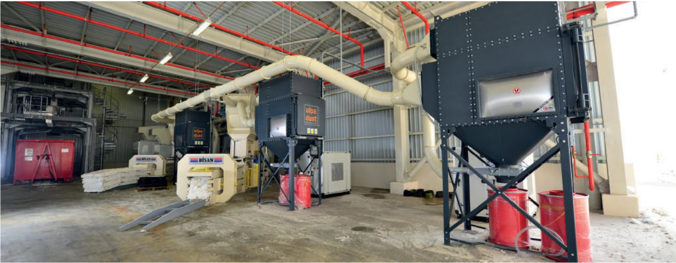
For the paper scrap & trim transport systems dust collection systems are very essential for optimum working conditions. While paper, carton box can have varied sizes to be filtered, especially tiny dusts may lead to explosion and/or fire. In addition to these, dusts can lead to serious respiratory problems such as asthma, bronchitis, allergic reactions, conjunctivitis and shortness of breath.
