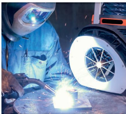
The method of vacuuming from the tool is the most effective method for removing dust and fume from the environment. Some applications, the dust should be held with downdraft table, slot vacuum, etc. Also this environments need to be supported with the right filtrations systems which to supply minimum ACH for the enclosed space.
