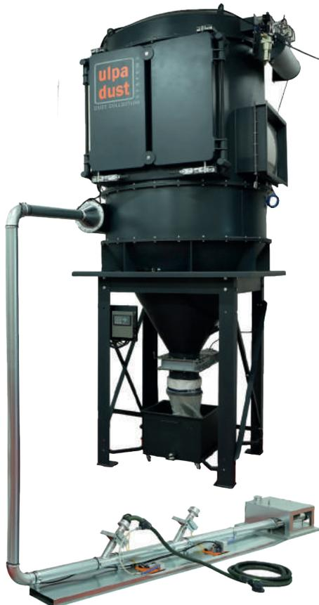
The method of vacuuming from the tool as it's the source which is the most effective method for removing dust from the environment. However, in some applications, the dust should be held with downdraft table, slot vacuum or other tailor made solutions. Also, this environment need to be supported with the right filtrations systems which to supply minimum ACH for the enclosed space.
