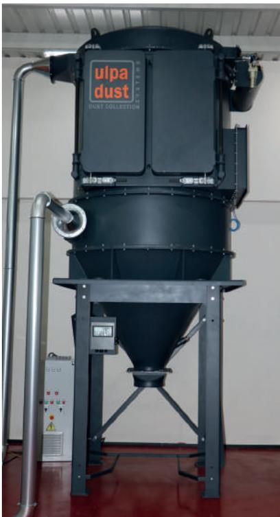
Pharmaceutical dust is highly toxic and explosive. Ulpadust can give solutions with its certified products and systems which are compatible with ATEX legislation.
