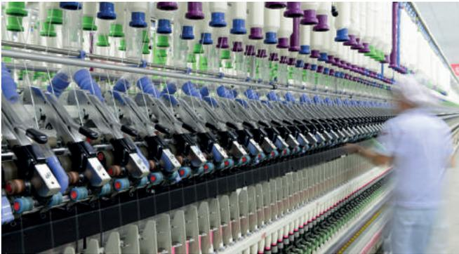
In modern textile plants with high speed machines, its only possible to produce and keep the quality high by having good air-conditioning systems maximum productivity is obtained from the system by keeping the humidity and temperature constant at a required level while keeping the working environment clean always.
